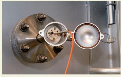
In-situ calibration method\*, without dismantling the sensor: simple and easy to set up.
